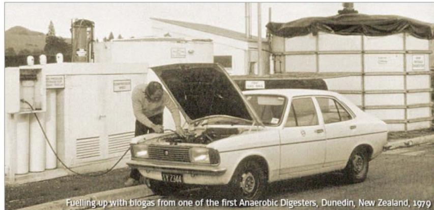
Fuelling up with biogas from one of the first Anaerobic Digesters, Dunedin, New Zealand, 1979
